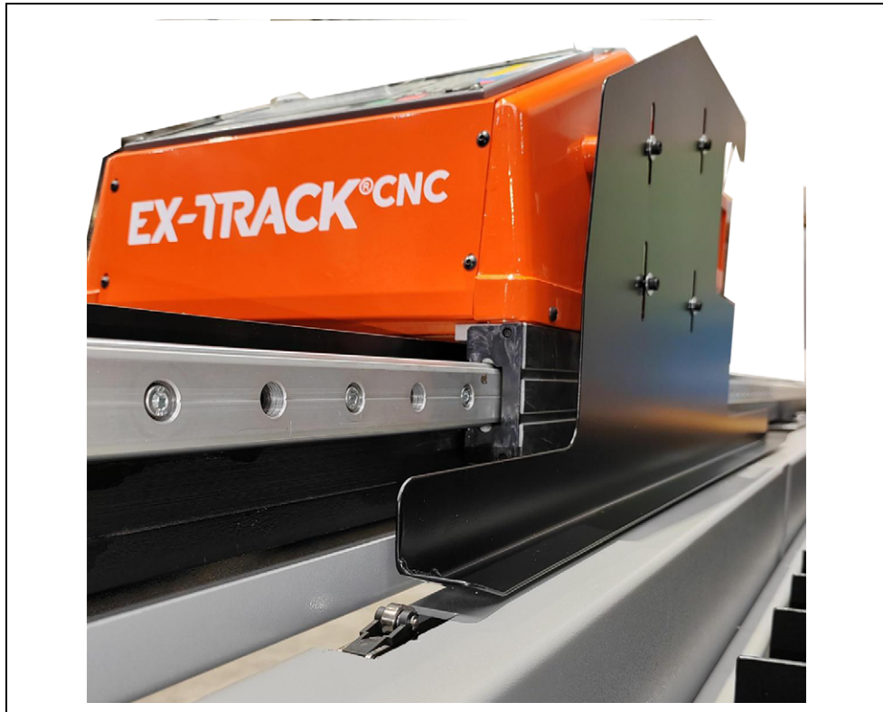
Fig. 5 EX-TRACK CNC with activation rail
