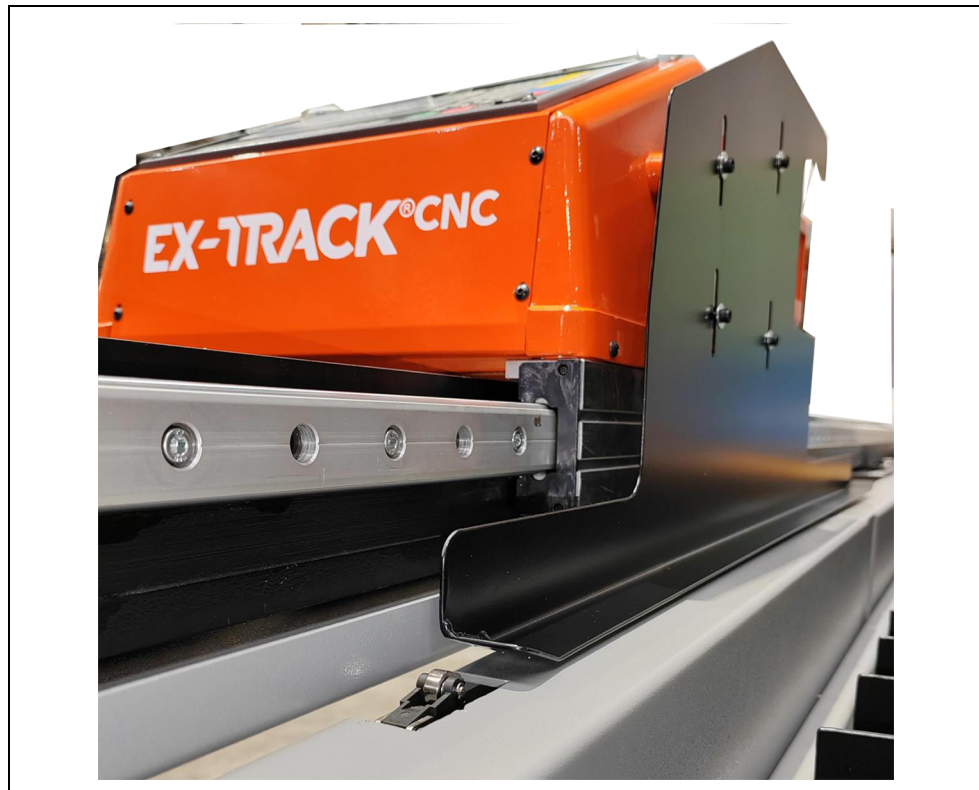
Fig. 5 EX-TRACK CNC with activation rail
